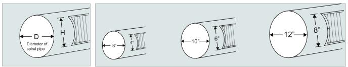
The height of the diffuser needs to be 4" less than the pipe diameter.
