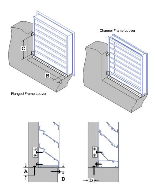
Louver being installed with angles or angle clips should have fasteners located as per the following chart:
